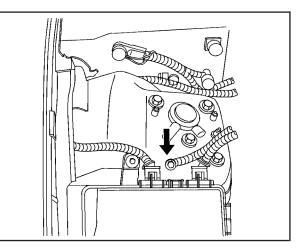
Your vehicle has a remote negative (–) ground location, as shown in the illustration. It is located between the battery and the underhood fuse block. You should always use this remote ground location, instead of the terminal on the battery.
